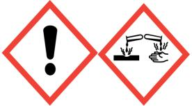
Wet concrete/floor screed is a strong alkali Warning, Contact with eyes may cause eye irritation and serious eye damage.
